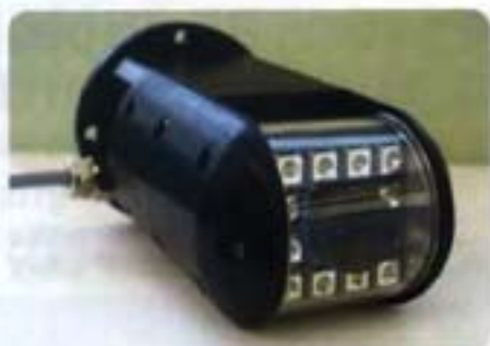
The camera head used for operational control of the robot during cutting works.
