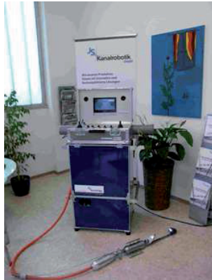
The JS Kanalrobotik curve robot alongside its control unit and power pack as displayed in full at a recent trade fair.
